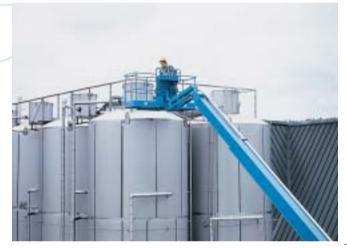
**S-85 Out-and-Up Articulating Jib Boom** This special option gives you an additional 1.52 m (5 ft) of horizontal reach for a total of 23.4 m (77 ft). The S-85 jib gives you flexibility too –  $135^{\circ}$  of working range. You not only access  $75^{\circ}$  above horizontal, but you can get to  $60^{\circ}$  below horizontal.
