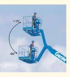
S-45 Out-and-Up Articulating Jib Boom This special option gives you an additional 1.52 m (5 ft) of horizontal reach for a total of 11.2 m (36 ft 8 in). The S-45 jib boom gives you flexibility too – 135° of working
